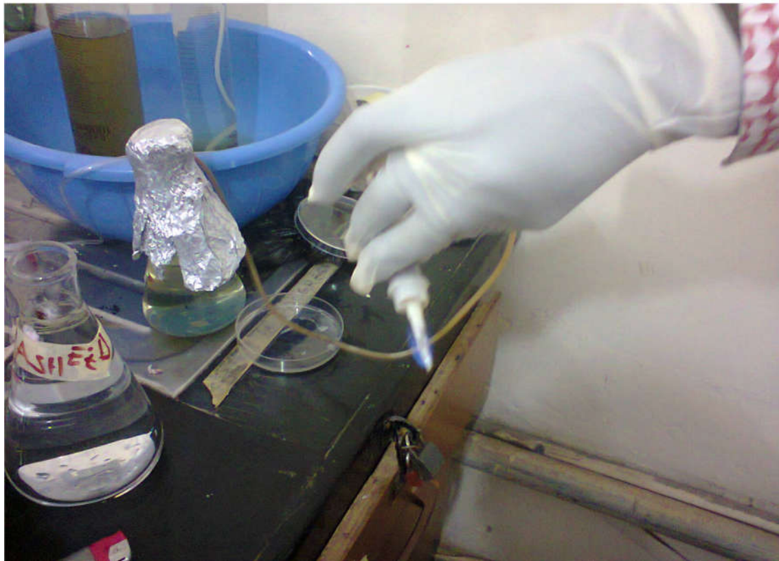
Plate 1. Combustibility of biogas (methane) produced from rice husk.
